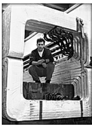
DONUT spokesman Vittorio Paolone, University of Pittsburgh, poses inside the magnet used to eliminate charged particles from the neutrino beam. (www.fnal.gov)
