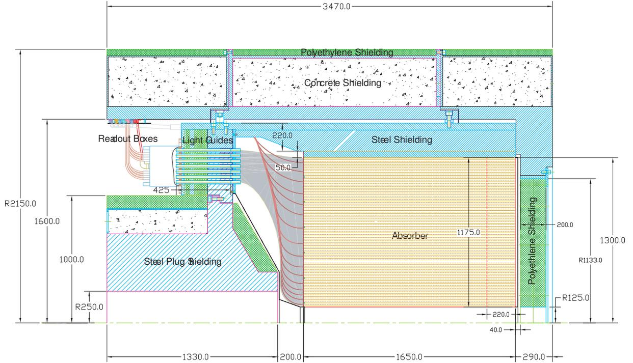
Figure 1: Cross-sectional view of the HF, where  $r$  increases vertically and  $z$  increases to the left (i.e., showers enter from the right). Steel absorber plates and other shielding is shown. Photomultipliers are located in the readout boxes. The vertical dashed red line marks the end of the short fibers.
