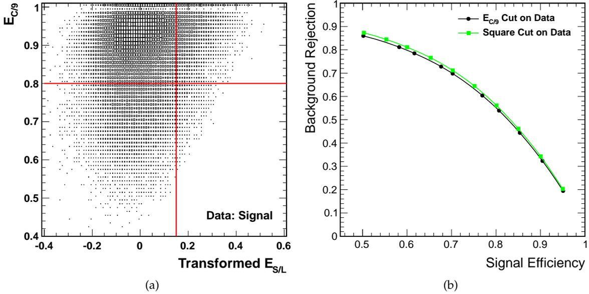
Figure 11: (a)  $E_{C/9}$  vs.  $E_{S/L}^{\text{cor}}$  with example square cut-lines for “Data: Signal.” (b) Comparison of the square cut and the  $E_{C/9}$  cut on data, which turn out to have nearly identical effects.
