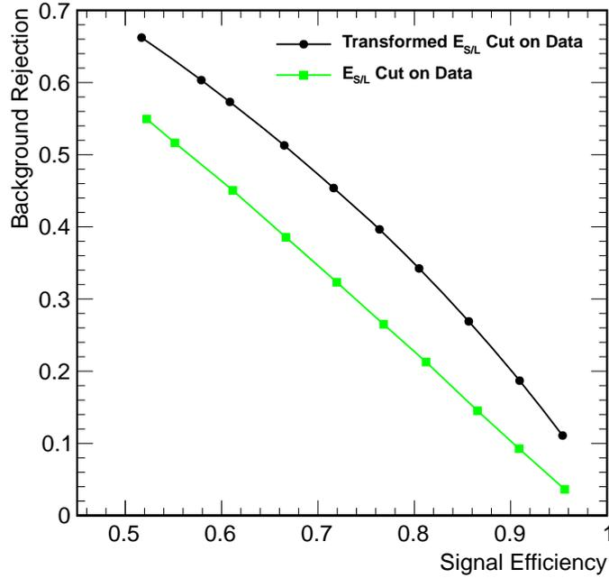
Figure 9: Comparison of the  $E_{S/L}$  and  $E_{S/L}^{\text{cor}}$  cuts. For each value of signal efficiency, the  $E_{S/L}^{\text{cor}}$  gives greater background rejection.
