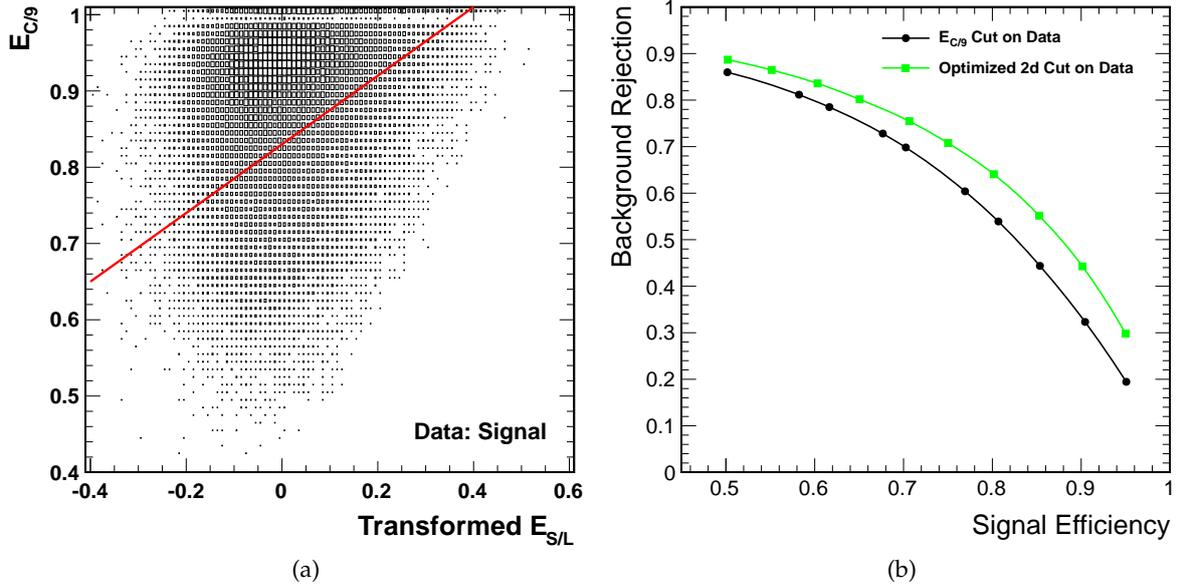
Figure 13: (a)  $E_{C/9}$  vs.  $E_{S/L}^{\text{cor}}$  with an example 2d cut-line for “Data: Signal.” (b) Comparison of the new 2d cut and the  $E_{C/9}$  cut on data, where it is clear that the new 2d cut offers an improvement in background rejection.
