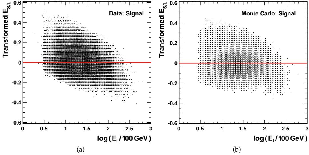
Figure 7: Plot showing  $E_{S/L}^{\text{cor}}$  vs.  $\log(E_L / 100 \text{ GeV})$  for (a) real signal and (b) simulated signal. After the transformation the distributions are flat, and a line fit to the dense regions of events would coincide with the  $x$ -axis.
