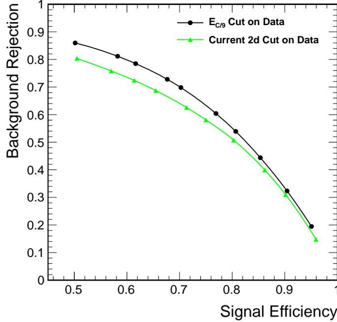
Figure 10: Comparison of the transverse and current two-dimensional cuts. For the tight cuts shown here,  $E_{C/9}$  is more effective than the cut in equation (3).
