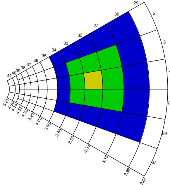
Figure 2: Three adjacent wedges of HF, each spanning  $\Delta\phi = 20^\circ$ , shown in  $r\phi$ -space. Indices on the upper and outer edges are called  $i_\eta$  and  $i_\phi$ , respectively. The values along the lower edge denote the  $\eta$ -values of the cell boundaries. As introduced in Section 4.3, the shading depicts the seed cell (in yellow),  $3 \times 3$  region (green + yellow), and  $5 \times 5$  region (blue + green + yellow) of an electromagnetic cluster.
