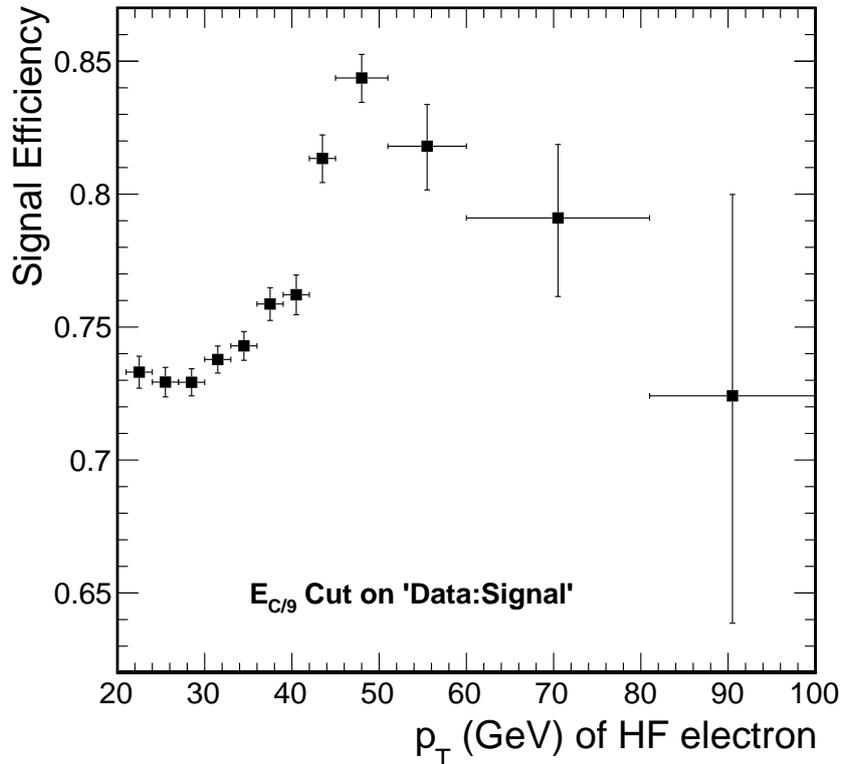
Figure 14: Plot of modified signal efficiency versus transverse momentum of the HF electron. The efficiency depends of  $p_T$ , showing that an improvement can be made in the transverse shower-shape variable.
