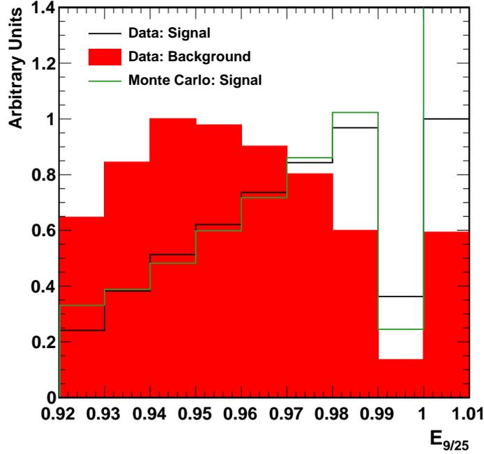
Figure 3: Histogram depicting  $E_{9/25}$  for data and simulation. We see reasonable agreement between data and simulation, disregarding the rightmost bin. The Monte Carlo sample has many more events with  $E_{9/25} = 1$  than does “Data: Signal” because we have not re-weighted the simulation, which was produced with less-pileup.
