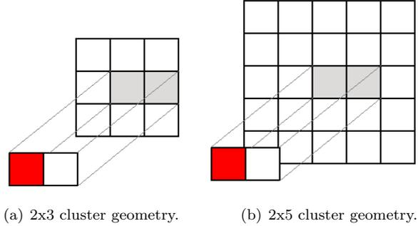
Figure 3: Cluster geometries tested in this simulation. ECAL towers are pictured in the foreground, while HCAL towers are shown in the background. The ECAL seed tower is shown in red.
