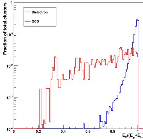
Figure 5: A plot of the fraction of total events vs. ECAL purity at 20 pileup and no HCAL segmentation, with a 2x5 cluster geometry.
