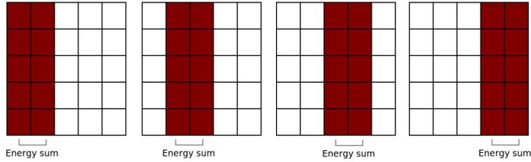
Figure 4: Electron-photon triggering algorithm being applied to an ECAL trigger tower.
