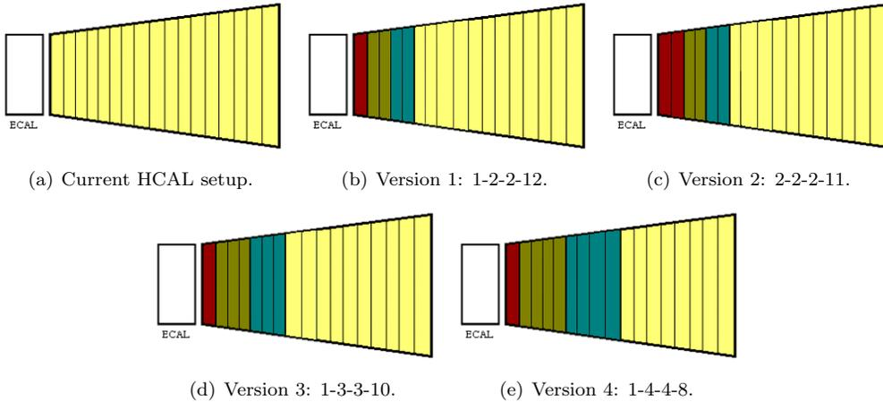
Figure 2: HCAL segmentations considered in this simulation for the SLHC upgrade. The segments are grouped by color.
