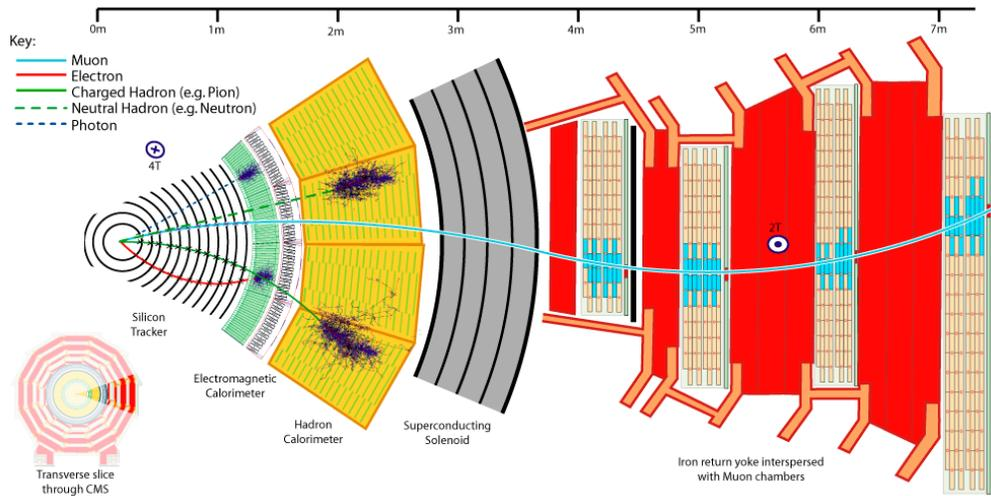
Figure 1: A slice of the CMS detector from a beam-axis perspective.
