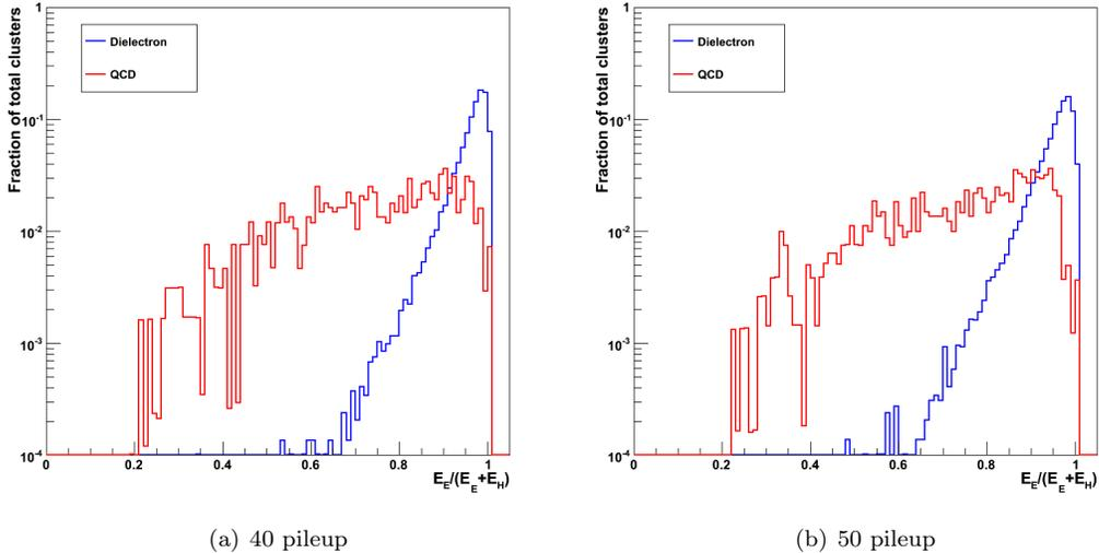
Figure 6: Plots of the fraction of total events vs. ECAL purity at higher pileup numbers and no HCAL segmentation, with a 2x5 cluster geometry. These plots simulate the current detector performance at SLHC-like pileup numbers.
